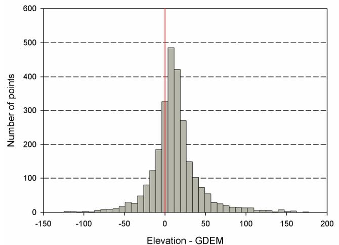
Figure 2. Histogram of control points heights minus GDEM heights. Some statistics for this distribution: D of Kolmogorov-Smirnov test=0.1165;  $p < 0.01$ , Lilliefors- $p < 0.01$ ; number of elements=2592; Mean=12.33; Standard deviation=30.62; Maximum=177.47; Minimum=-124.45 and Shapiro-Wilk test  $W=0.91$ ;  $p=0.00$ .
