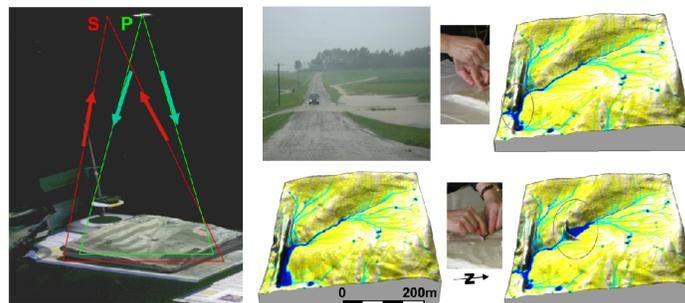
Figure 6. Tangible Geospatial Modeling System: a model is scanned to create a DEM while GIS data are projected over the model; simulation of overland flow exploring impact of road breach and a check-dam on flow pattern.
