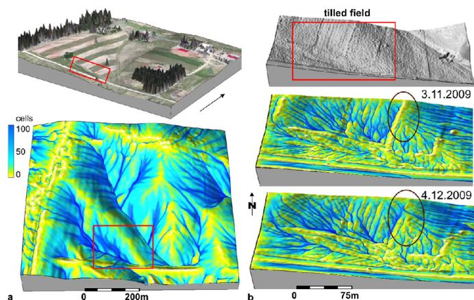
Figure 5. Flow tracing in a small watershed that includes tilled field modeled (a) at 1m resolution from DEM derived from airborne LiDAR data, and (b) at 0.20 m resolution from DEMs derived from terrestrial laser scanner.
