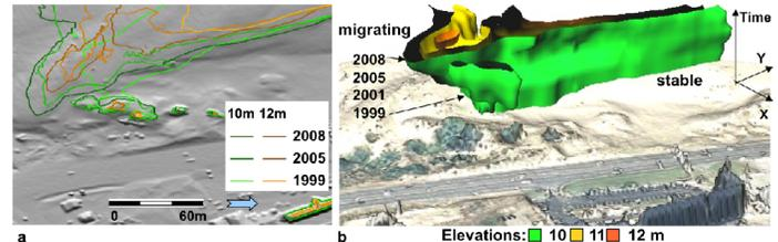
Figure 4. Elevation evolution in space-time cube: (a) limited, but hard to interpret set of contours  $z=10,12$  m for the years 1999, 2005, 2008, (b) space-time isosurfaces derived from 1999, 2001, 2004, 2005, 2007, 2008 point data, equivalent to  $z=10,11,12$  m contours stretched in the vertical time dimension.
