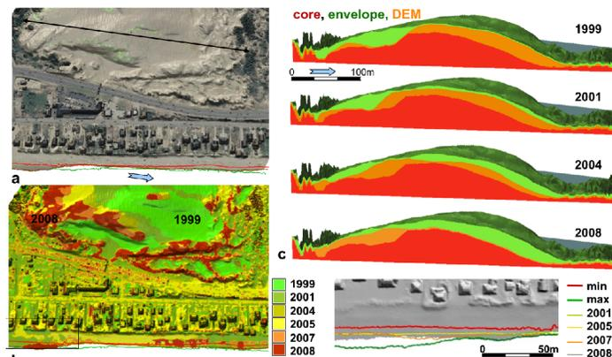
Figure 3. Raster-based analysis of coastal terrain dynamics: (a) 2008 DEM with orthophoto and shoreline band, (b) time of elevation maximum map draped over a 2008 DEM, (c) cross-section through core, envelope and migrating dune surfaces. Inset shows detail of shoreline band with actual shoreline positions.
