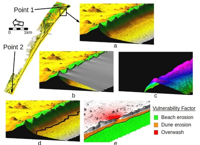
Figure 1. Coastal feature extraction using the LCP method: (a) DEM with extracted dune ridge, (b) DEM with sheet anchored at dune ridge and shoreline, (c) surface showing the elevation difference  $\Delta z$  between the DEM and the sheet, (d) dune ridge and dune toe, (e) vulnerability factor draped over DEM.
