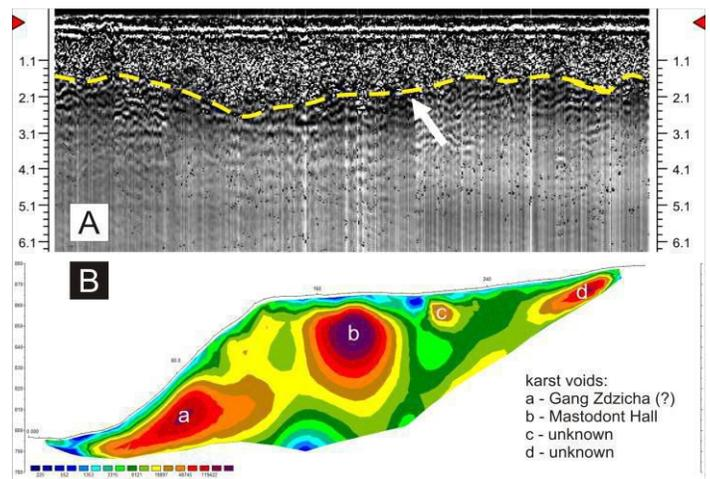
Figure 3. Examples of crystalline limestones imaging by ground penetrating radar (A) and 2-dimensional electrical resistivity tomography (B) – profile 1. Yellow line shows a boundary between solid and weathered rocks.
