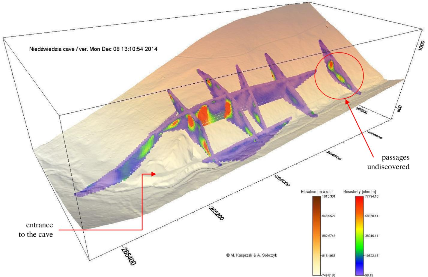
Figure 4. 3-dimensional image of karst voids detected by electrical resistivity tomography in the Kleśnica valley. Fields in ERT profiles, marked with “warm” colors, indicate a location of high resistivity areas – karst voids.
