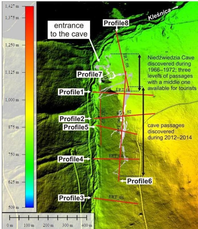
Figure 1. Electrical resistivity tomography profiles in the Kleśnica valley.
